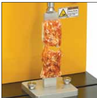
TA-PTF F M Pizza Tensile Fixture quantifies cooked pizza firmness by measuring the tensile force and deformation distance to break sample.
