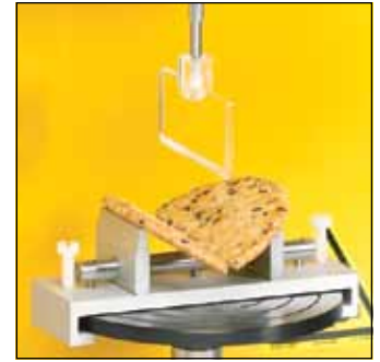
TA-JTPB F Small scale version of Three Point Bend Fixture is used with TA7 blade from general probe kit. Rotary Base Table required.
